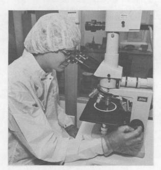
PAUL BASORE (6224) demonstrates one of the final steps of cell processing — inspection of the hair-thin metal interconnects, using a special microscope.
